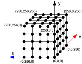
Fig. 4. An example of 3D LUT for 8-bit YUV input
