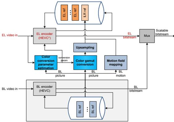
Fig. 3. Diagram of an SHVC CGS encoder
