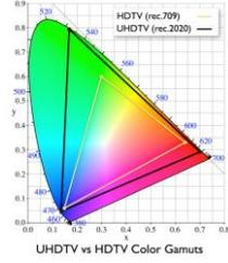
Fig. 1. BT.2020 and BT.709 color primaries comparison in CIE space
