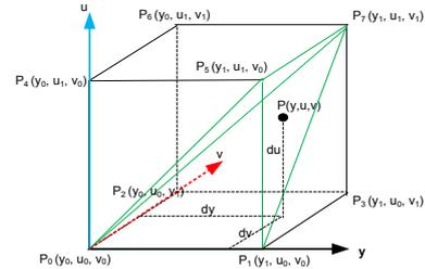
Fig. 5. Tetrahedral interpolation used in 3D LUT interpolation ([13])
