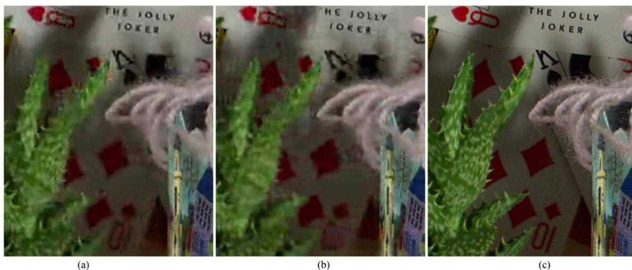
Fig. 8. Images cropped from 1080p sequence *Cactus*. (a) By ADS with the same horizontal and vertical ratio (PSNR Y 30.70 dB). (b) By H.264/AVC (PSNR Y 29.55 dB). (c) Original image.
