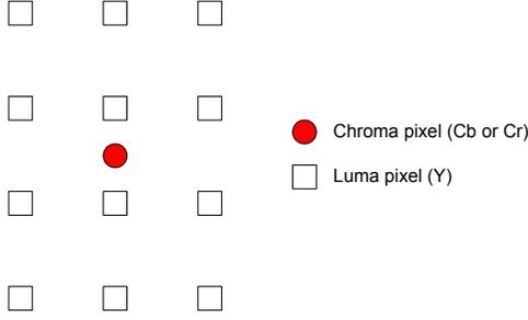
**Fig. 4 Relative Luma and Chroma pixel positions with 4:2:0 color subsampling format.**
