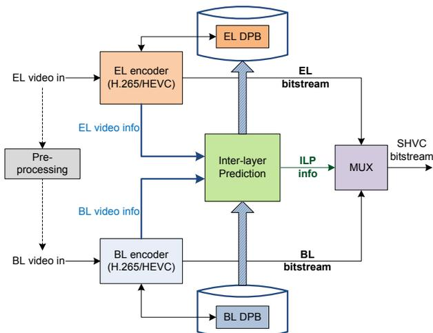
Fig. 1 Block diagram of two-layer SHVC encoder
