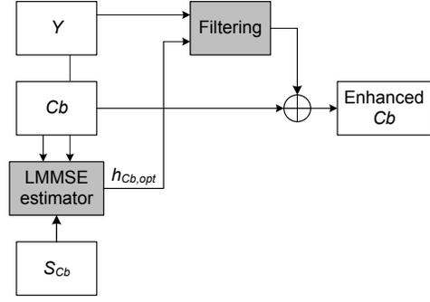
Fig. 3 Block diagram of the proposed CPCE scheme for Cb plane
